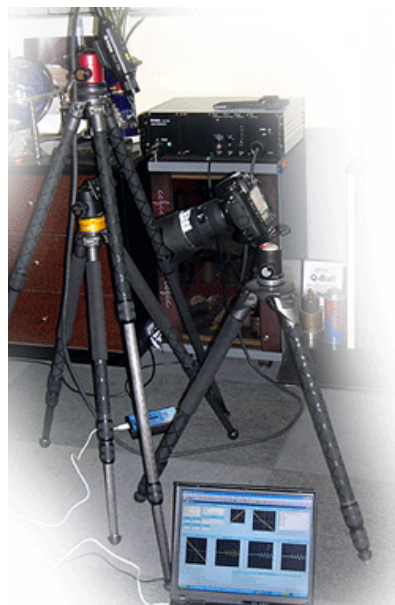
[Testing tripod-head vibration at the Markins office using Nikon D2H, laser vibrometer and data acquisition system]
